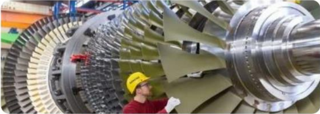
One 100MW gas turbine
